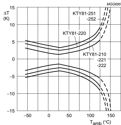
Fig.2 Maximum expected temperature error ( $\Delta T$ ).
