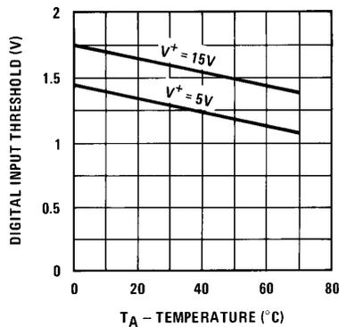
FIGURE 1. Digital Input Threshold vs Ambient Temperature
