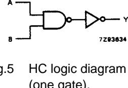
Fig.5 HC logic diagram (one gate).
