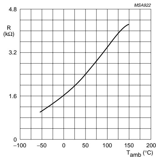
Fig.3 Sensor resistance as a function of ambient temperature; average values.
