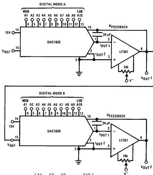
$$V_{OUT1} = -V_{REF} \left( \frac{A1}{2} + \frac{A2}{4} + \frac{A3}{8} + \dots + \frac{A10}{1024} \right)$$
