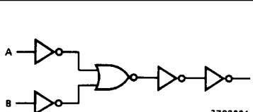
Fig.6 HCT logic diagram (one gate).
