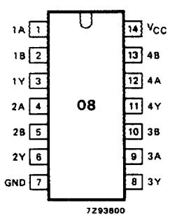
Fig.1 Pin configuration.
