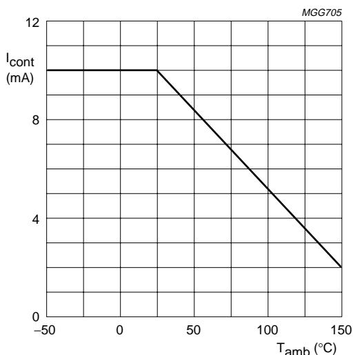
Fig.5 Maximum operating current for safe operation.
