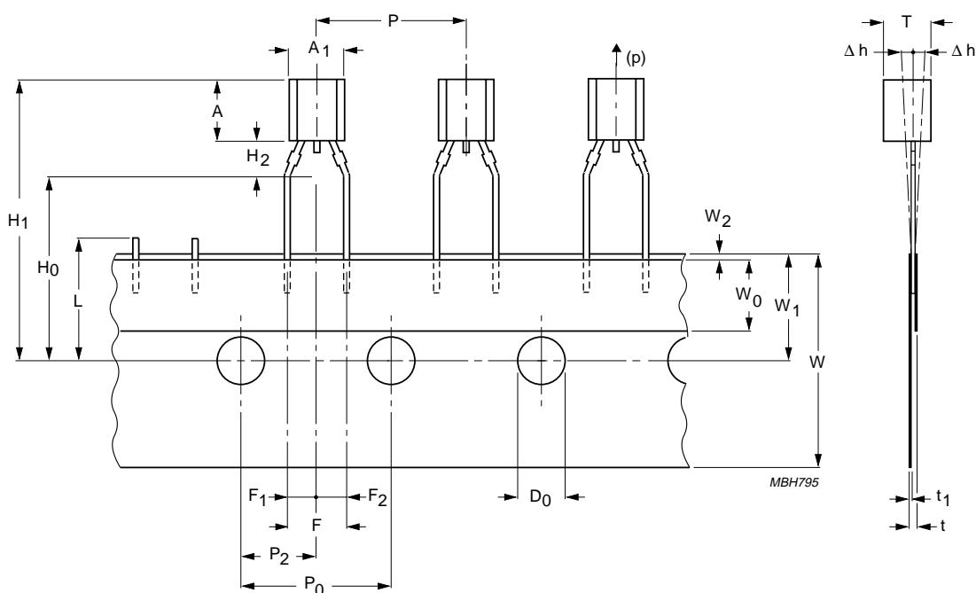
Fig.7 Configuration of bandolier.
