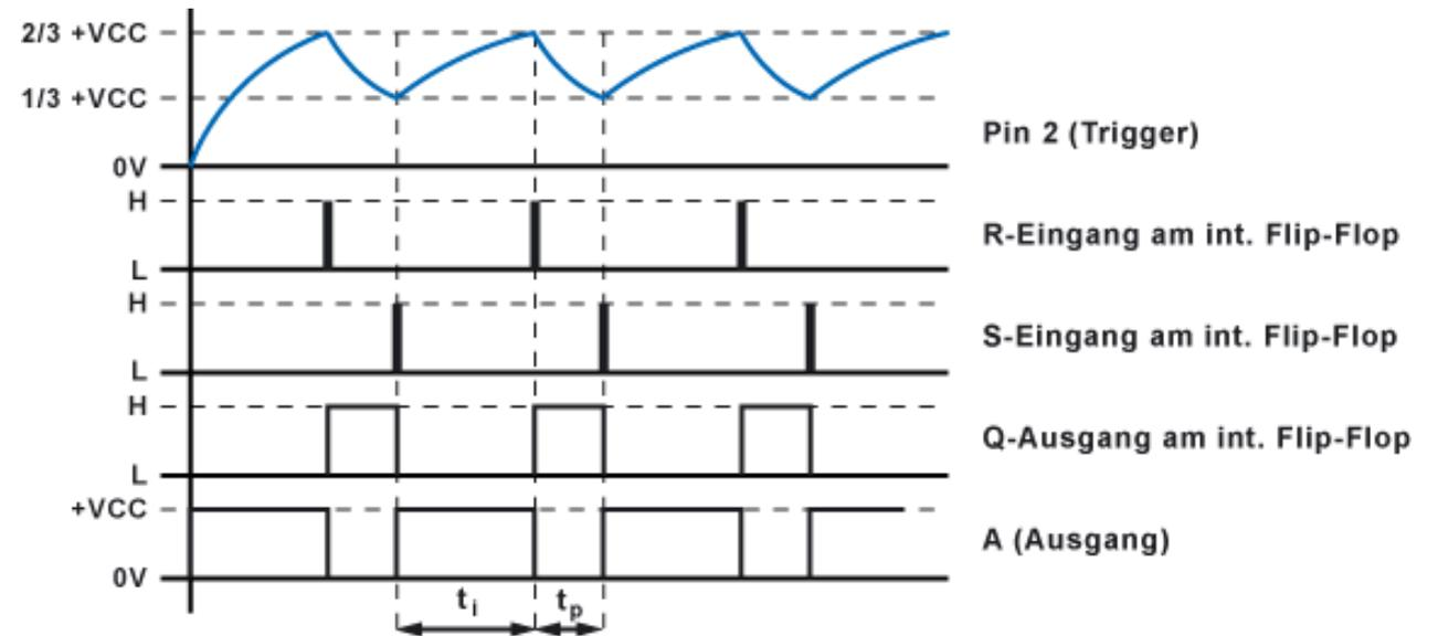
$$f = \frac{1}{(R_1 + 2R_2) * C * \ln(2)} ; t_{high} = (R_1 + R_2) * C * \ln(2) ; t_{low} = R_2 * C * \ln(2)$$
